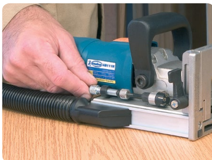
Quick adjustment of different grooving depths.
