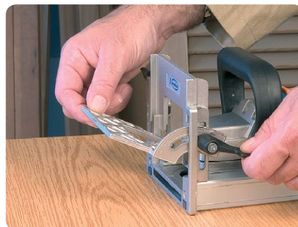
Angle and height adjustable front fence with graded scale.
